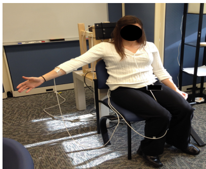
Figure 4: Subject positioning for motion analysis. Four sensors were attached to the subject and secured with a pre-wrap tape.
