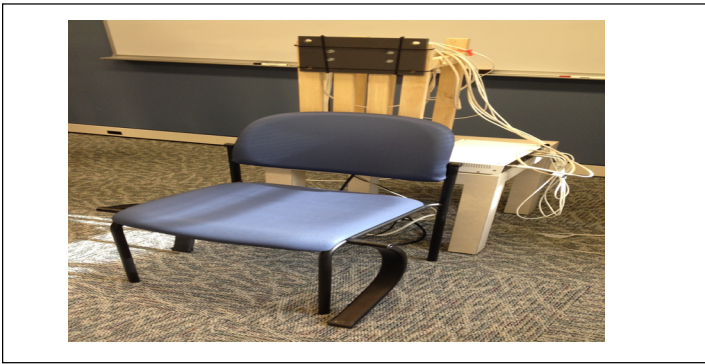
Figure 3: Motion analysis apparatus consisting of the transmitter mounted to a rigid base and a chair for the subjects.the five subjects in this study who were all treated non-operatively at our institution.
